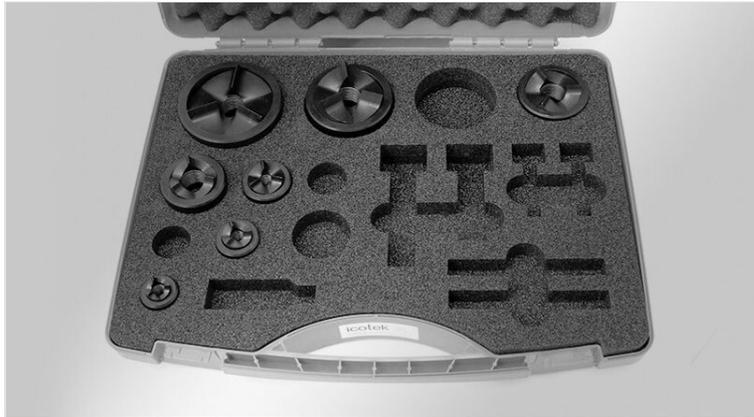
Self-centering knockout punches for stainless steel or mild steel, aluminium and plastic walls with max. sheet thickness of 3 mm. Punches for cut-outs M16, M20, M25, M32, M40, M50 and M63. Cut-outs for icotek split cable glands and round cable entry plates can be punched.
